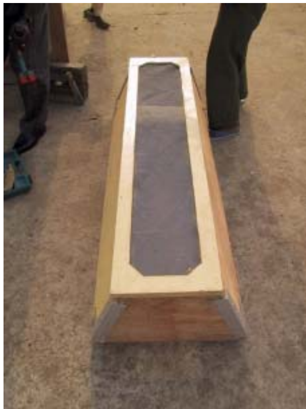
Figure 3.5. The extension box of the drying bed.
