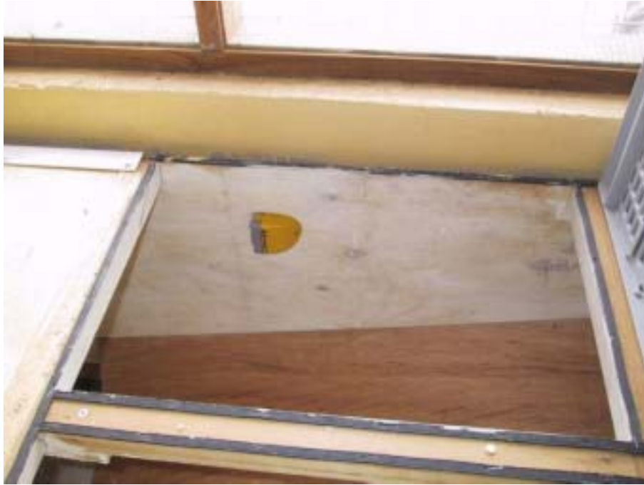
Figure 2.14. The combined temperature/humidity sensor in the pressure chamber.
