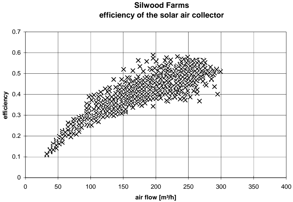
Figure 2.35. The efficiency of the collector at Silwood Farms as a function of the air flow rate through the system (based on total radiation on the collector).
