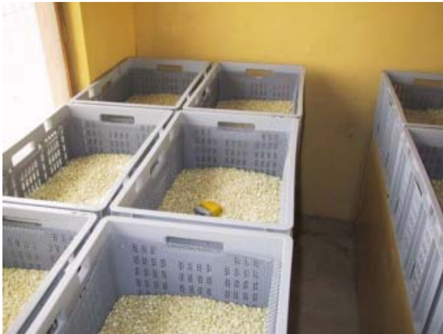
Figure 2.15. The combined temperature/humidity sensor located on top of the maize in one of the trays for measuring the condition of the air leaving the drying bed.
