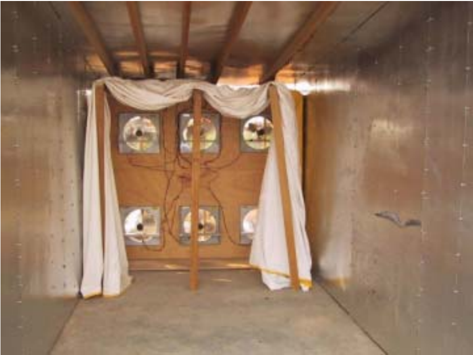
Figure 4.3. The pressure chamber of the forced open-air dryer with fans and the tarpaulin.
