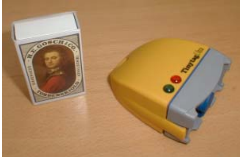
Figure 2.11. Picture of a Tinytag for combined measuring of the air temperature and the air relative humidity together with a Danish matchbox.
