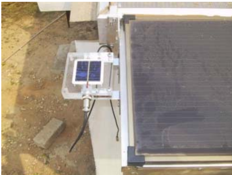
Figure 2.19. The PV-pyranometer of the measuring system.
