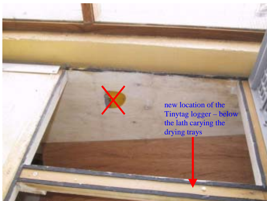
Figure 2.20. The new location of the combined temperature/humidity sensor in the pressure chamber.
