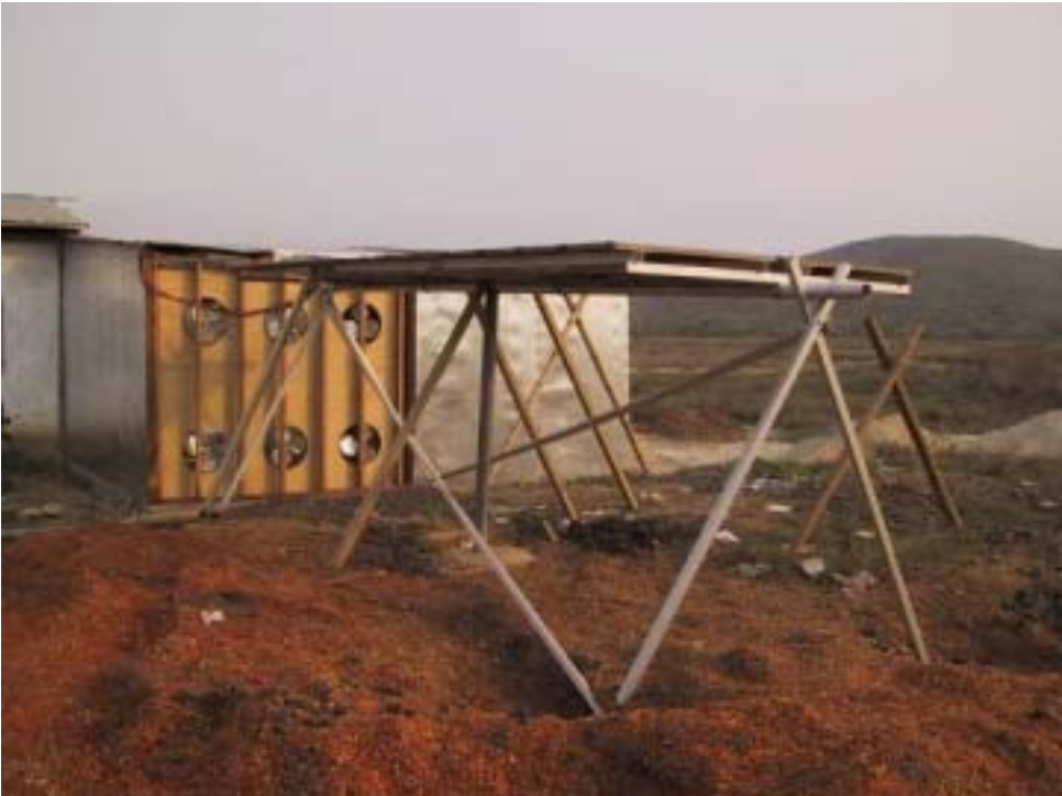
Figure 4.4. The pressure chamber of the forced open-air dryer and the PV-panel in front seen from the south.
