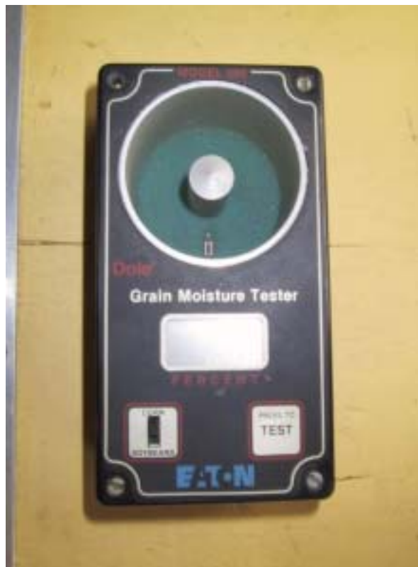
Figure 2.8. The instrument for measuring of the water content present at the farm.
