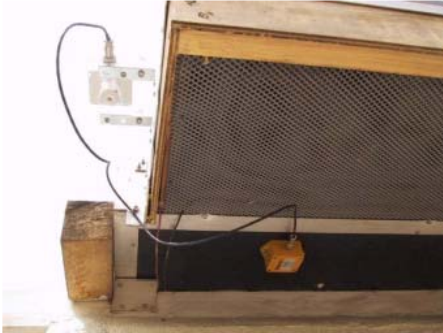
Figure 2.18. The Tinytag connected to the pyranometer.
