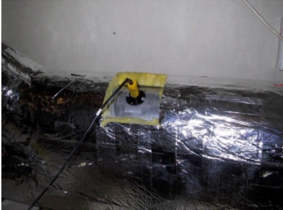
Figure 3.7. One of the applied VentCaptor air speed sensors.
