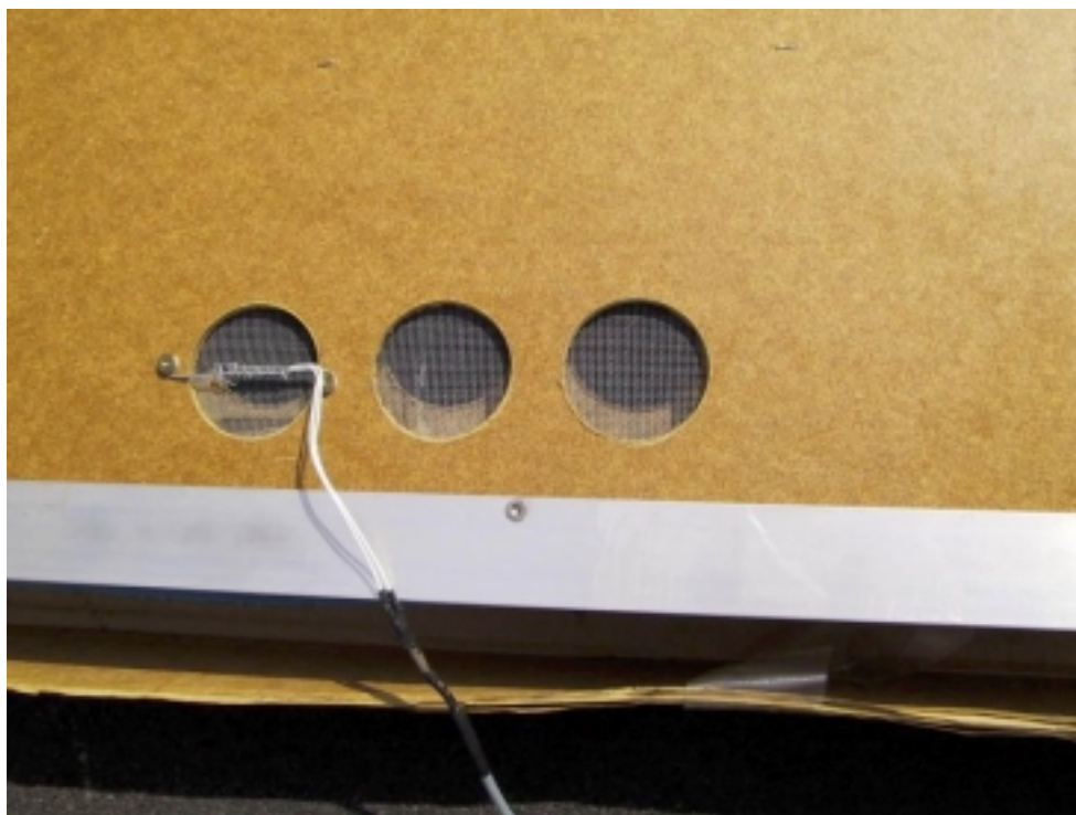
Figure 3.6. The inlet temperature sensor for the single solar air collector with fibre cloth absorber.
