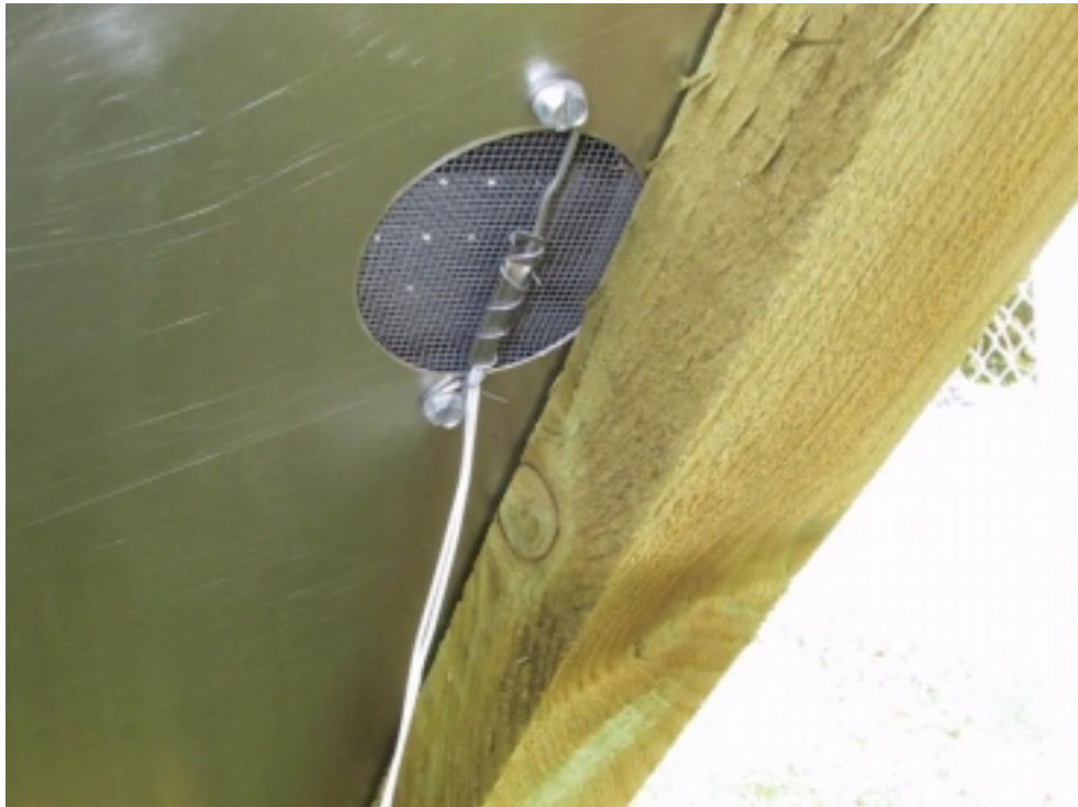
Figure 3.5. The inlet temperature sensor for the single solar air collector with perforated metal absorber.
