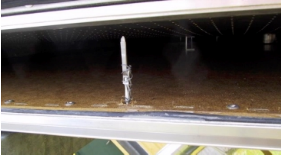
Figure 3.10. One of the two air temperature sensors in the connection between the connectable solar air collectors in the air stream behind the absorbers.
