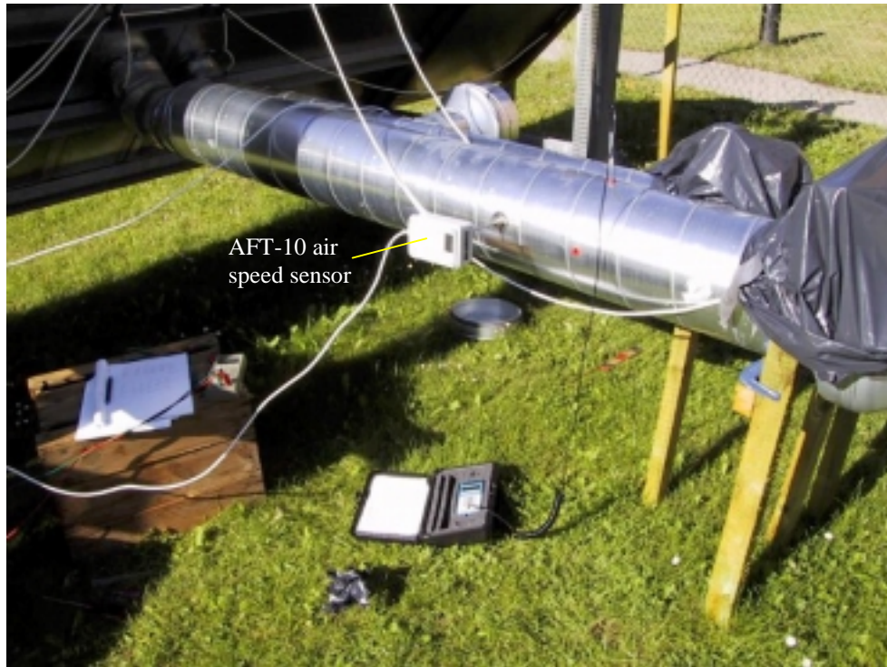
Figure 3.11. Envic AFT-10 air speed sensor and set-up for calibration of the air speed sensor.
