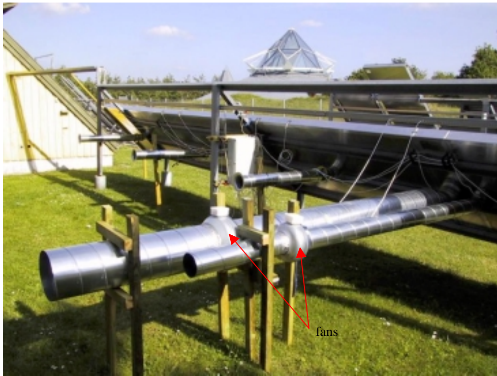
Figure 2.18. The fans for dragging air through the connectable solar air collectors and the single solar air collector with perforated metal absorber. The different measuring features shown on the picture will be discussed in the following chapter.
