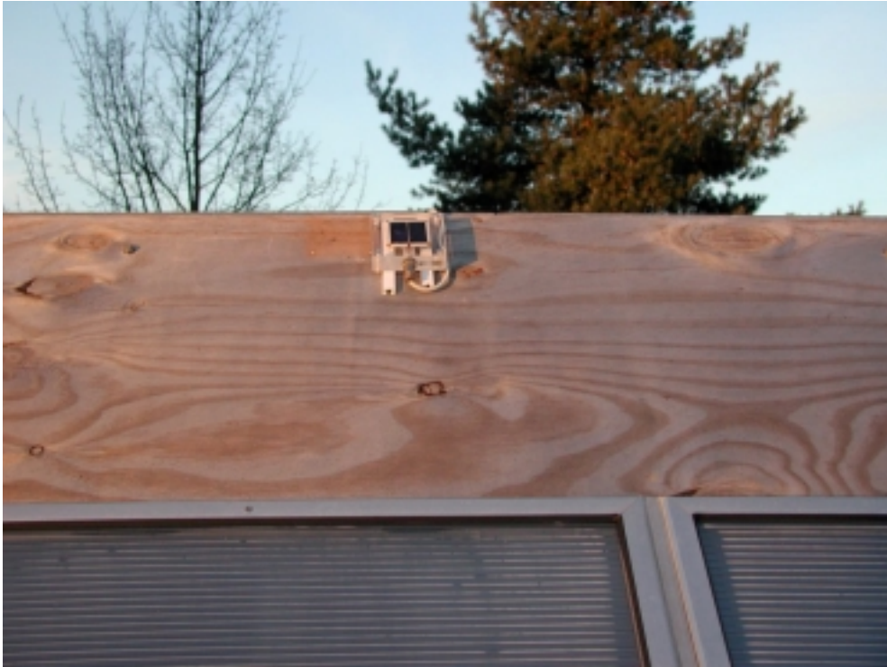
Figure 3.15. The applied PV pyranometer mounted above of the connectable solar air collectors.
