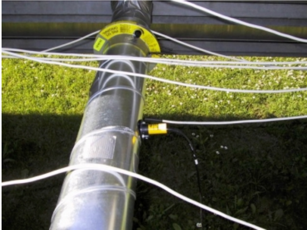
Figure 3.13. Example of an VentCaptor air speed sensor in the air intake of one of the connectable solar air collectors.
