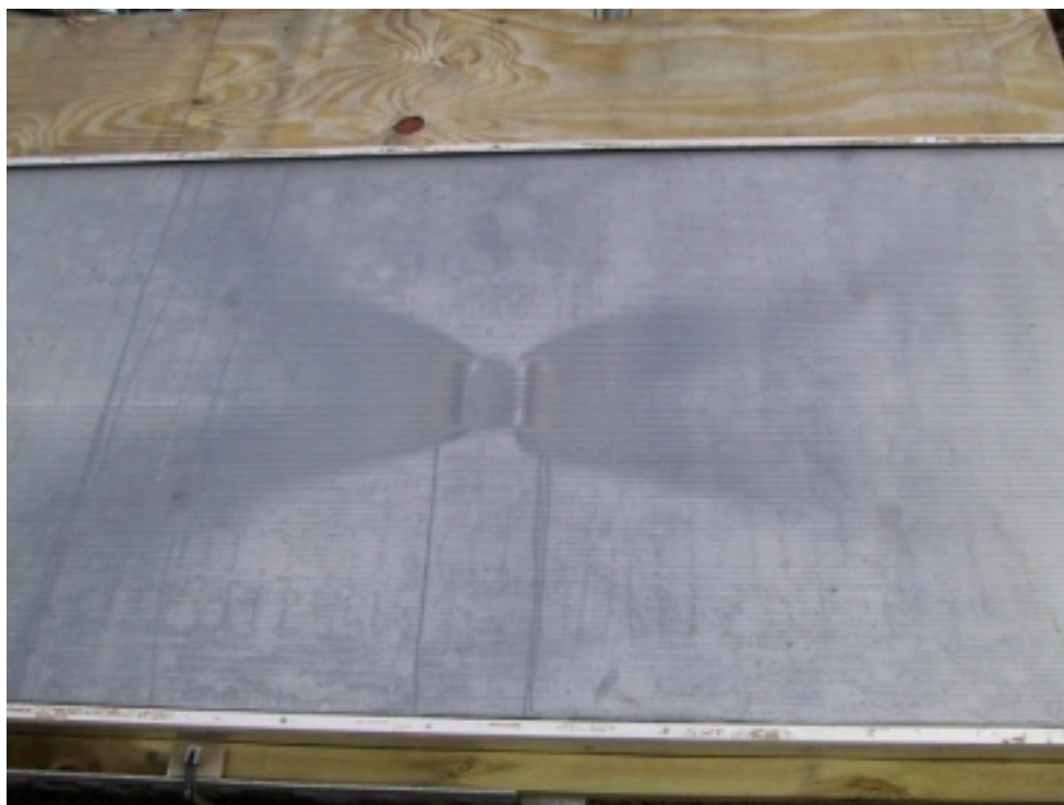
Figure 4.9. The air flow path in one of the connectable solar air collectors.
