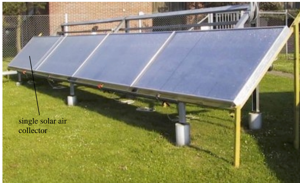
Figure 2.13. The 9.22 m 2 solar air collector consisting of three connectable collectors of each 2.98 m 2 and a manifold collector of 0.28 m 2 . At the far back of the collector array is seen the single collector also with a perforated metal absorber.
