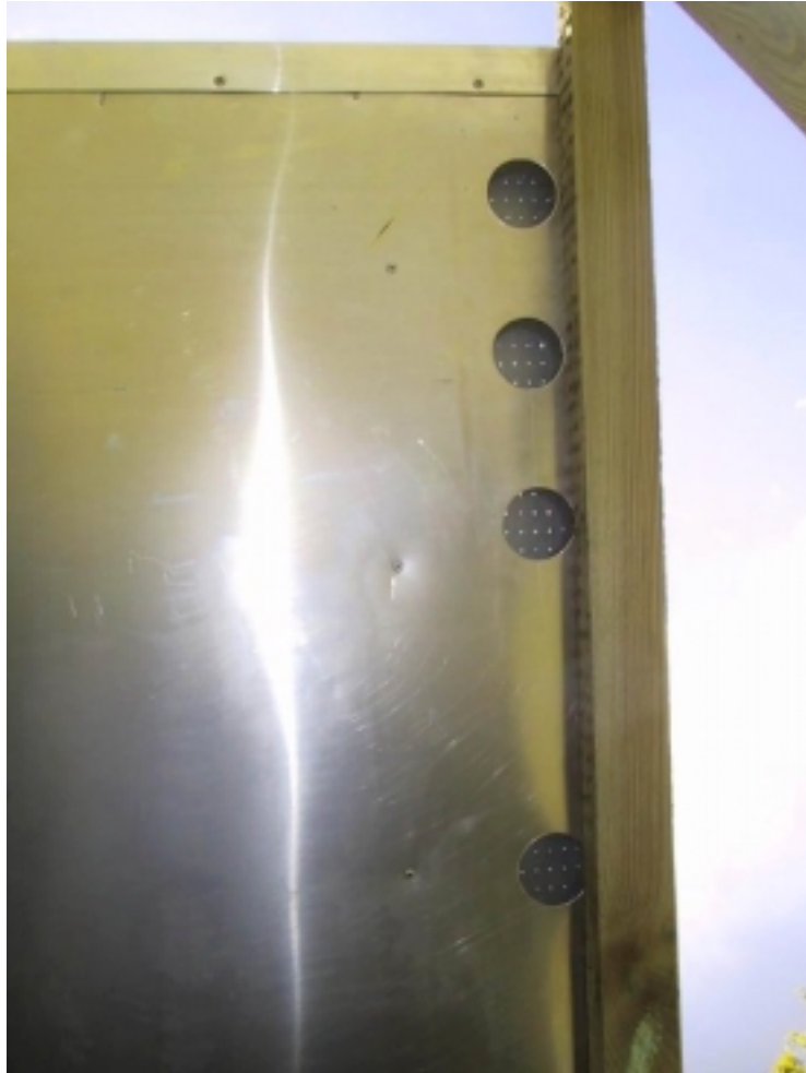
Figure 2.15. The middle and three top air intakes of the single solar air collector with perforated metal absorber.
